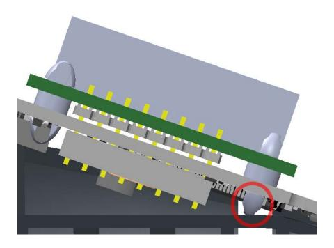
It's helpful to rotate the two lower LCD standoffs as shown, so the latch clip is horizontal. There is a slight interference with the top of the battery compartment on the bottom case, and if the standoffs are properly oriented it will make final assembly easier.
