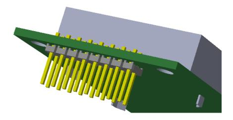
Solder the LCD header as shown, with the spacer flush to the underside of the LCD PCB. There is not much clearance at final assembly, so there can't be gaps between the spacer and the PCB.
